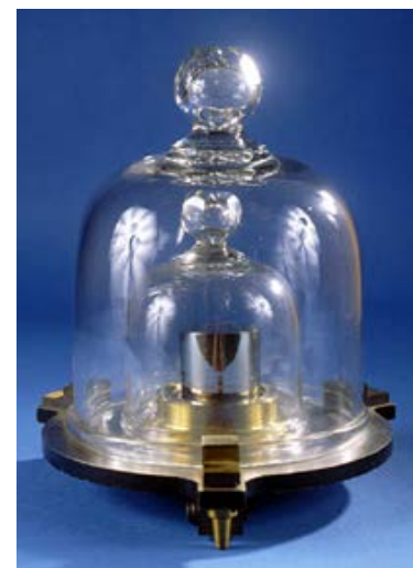
Figure 1.8 The Kilogram. The standard for the kilogram is a platinum-iridium cylinder kept in a special vault in France. Source: Wikimedia ( https://commons.wikimedia.org/wiki/File:National_prototype_kilogram_K20_replica.jpg )
